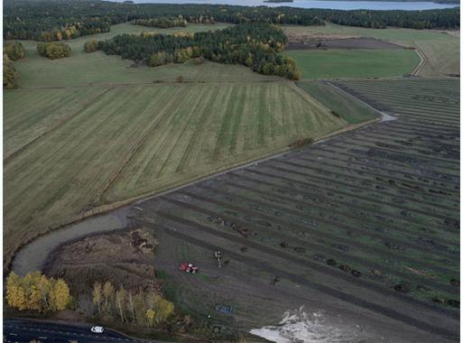
Structure liming, Filter ditches, and Phosphorus pond
