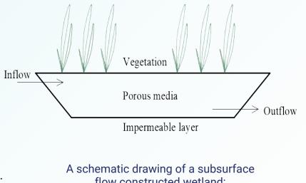
flow constructed wetland: 1. Inflow; 2. Impermeable layer, 3. Porous media, 4.Vegatation, 5 Outlet
